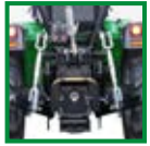
REAR LIFT WITH TWO CYLINDERS
