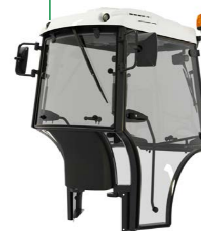
VISTA CLIMA 4 upright - Conical structure
